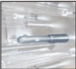
Measures UV intensity within the reactor. Automated cleaning system prevents fouling of the photodiode sensor's quartz sleeve.
