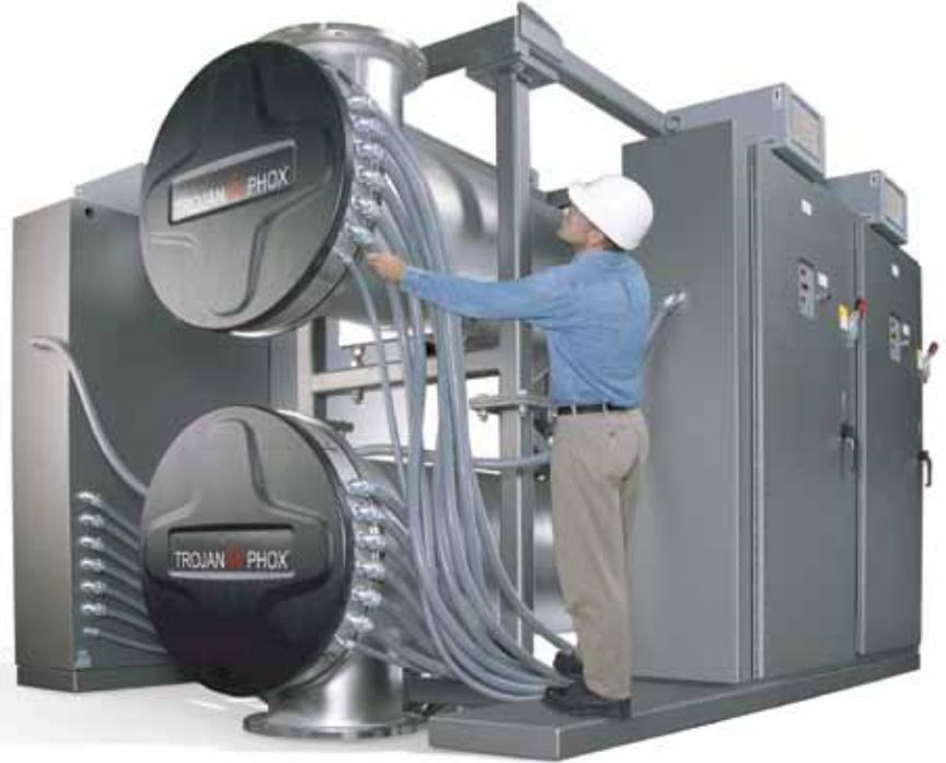
*Trojan's leadership is demonstrated by the patent-pending TrojanUVPhox™ that is being used to cost-effectively treat NDMA and other contaminants in drinking water and water reuse applications.*
