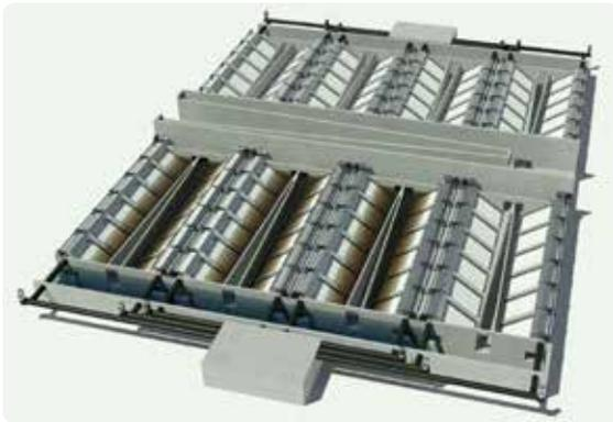
The Agua Prieta WWTP in Guadalajara, Mexico arranged modules to treat 350 MGD (55,200 m<sup>3</sup>/h) of wastewater using only 10,550 ft<sup>2</sup> (980 m<sup>2</sup>) of land. Primary settling tanks would have needed 215,000 ft<sup>2</sup> (20,000 m<sup>2</sup>) of land.
